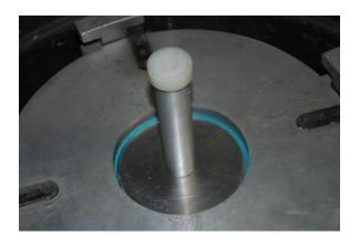
Machine after ring- molds are cast and distribution system removed. Machine may spin to allow cast material to congeal.
