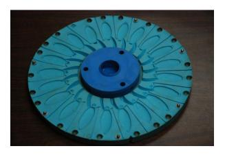
Vent attachment can be use to blow cooling for wax or exhaust for plastic.
