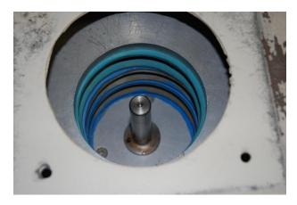
Typical ring-mold for fishing tackle with a single beehive inserted.
