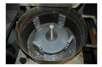
Machine with 3 12" ring-molds and distribution system installed ready for the cover plate.
